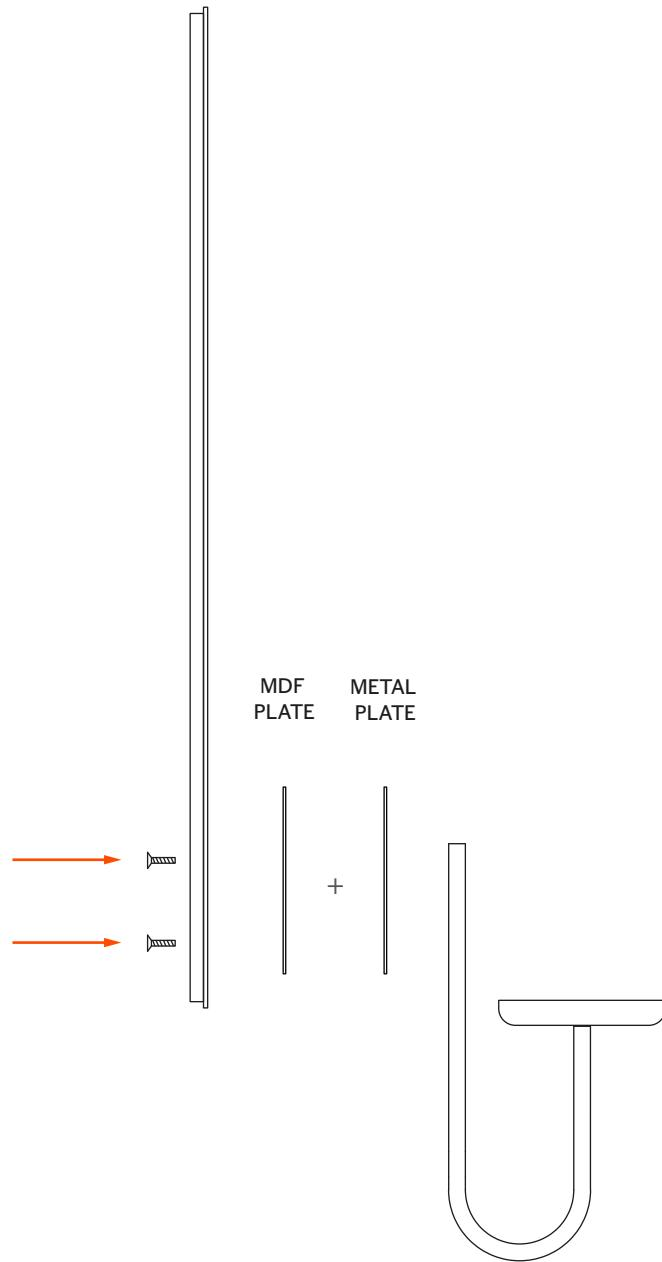
Avvitare lo specchio al tubo dal retro, incluse la piastra metallica e la sottile contropiastra in MDF. | Screw the mirror to the rear upper part of the metal tube, including the metal plate and the thin MDF plate in the middle.
